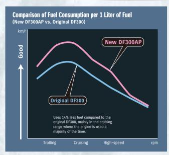
Data used in the graphs were obtained through in-house testing under uniformed conditions. Results will vary depending upon operating conditions (boat design, size, weight, weather, etc.)
