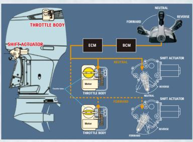
required for rigging and adjustment. The system offers precision control for single, twin or triple installation as well as dual station operation.
